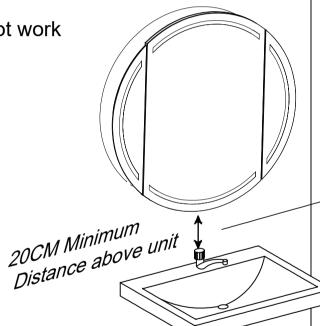
Ensure there is at least 20cm gap between the head of the sensor and the nearest obstacle
