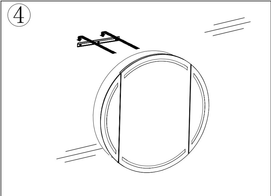
**5** The mirror cabinet is hung on the bracket, adjusting its left and right position, and open the mirror door. Then, mark the center of the round hole with a pencil.
